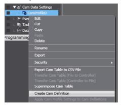
The cam definition is registered below the corresponding cam profile and displayed as follows: Cam\_definition\_name(Cam\_property\_variable\_name,Cam\_node\_variable\_name)
