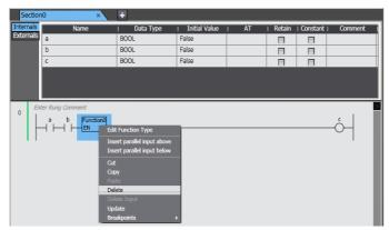
The selected function is deleted. Variables used as parameters are not deleted.
