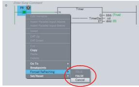
The forced value for the selected input or output is cleared and the forced value icon disappears. The TRUE/FALSE value does not change.
