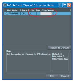
The size of the expansion areas is used to calculate the I/O refresh time for the specific CJseries Special Units.
