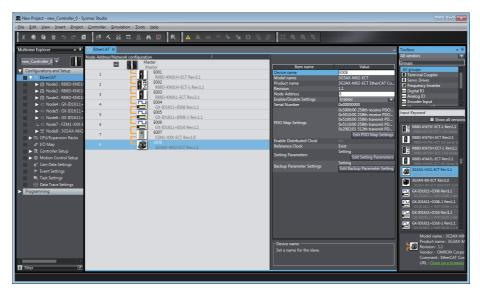
**3** Change the node address of the slave that you added to the EtherCAT Tab Page to the node address of the physical slave.
