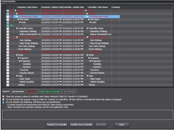
The CPU/Expansion Racks configuration information is downloaded from the Sysmac Studio to the Controller.
