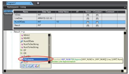
The selected function or function block instance is displayed. When you enter a left parenthesis, a description of the parameters is displayed.
