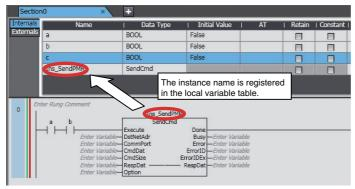
This completes the insertion of the function block. If you entered a new instance name, it is registered in the local variable table.
