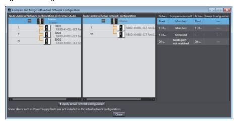
If there are slaves for which the comparison results do not match, correct the network configuration on the Sysmac Studio or correct the actual network configuration until the comparison results for all slave match.
