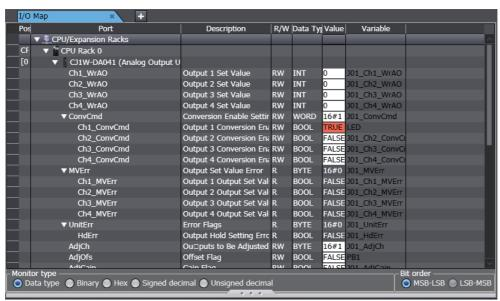
In the I/O Map, perform operations such as Set/Reset, present value change, and forced refreshing on output devices. Refer to 7-2-3 Changing Present Values and Set/Reset Using Forced Refreshing on page 7-23 for the procedures to execute Set/Reset, present value change, and forced refreshing in the I/O Map.
