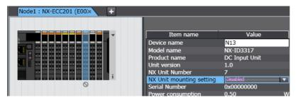
Change the setting to *Enabled* in the Unit setting item list to enable the Unit again.
