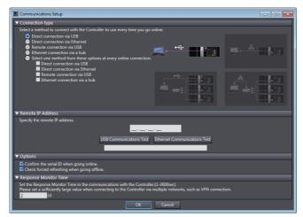
Select the connection method in the Connection Type Field. For a remote USB connection or Ethernet hub connection, enter the IP address of the Controller to which you need to connect in the Remote IP Address Field.
