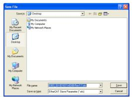
An EtherCAT slave parameter file with an .ets extension is saved.
