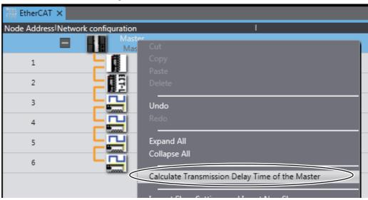
**2** The transmission delay times of PDO communications cycle 1 and PDO communications cycle 2 are displayed in the Output Tab Page.
