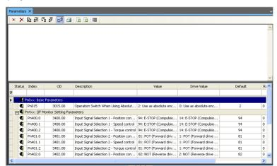
In this status, you can transfer just the parameters with differences to the Drive or transfer them from the Drive.
