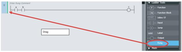
Method (2) Select the start of a rung and press the R Key. (Press the Shift + R Keys to insert a rung above the selected rung.)
