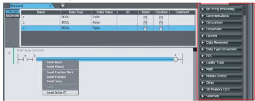
An inline ST box is inserted.
