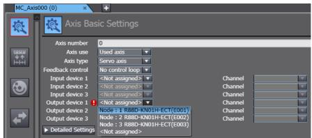
Refer to 5-2 EtherCAT Configuration and Setup for the procedure to set slaves.
