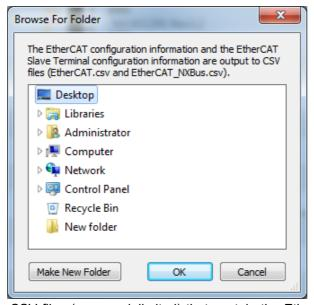
CSV files (comma delimited) that contain the EtherCAT network configuration information and the EtherCAT Slave Terminal configuration information are saved in the selected folder. Refer to 5-3-3 Exporting the EtherCAT Slave Terminal Configuration Information on page 5-32 for detailed information on the CSV file that contains the EtherCAT Slave Terminal configuration information.
