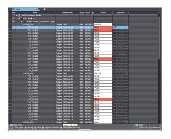
The data types that are given in the following table can be monitored in the I/O Map.
