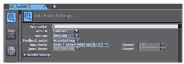
You must register the axis to use for the axis variable in advance under Configurations and Setup - Motion Control Setup - Axis Settings in the Multiview Explorer. When you register an axis, the variable for that axis is automatically registered as well.
