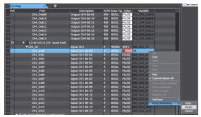
After you force the BOOL device variable to TRUE or FALSE, the value in the Value column in the I/O Map changes to TRUE or FALSE to reflect that change. An icon also appears by the BOOL device variable that represents its current forced value.
