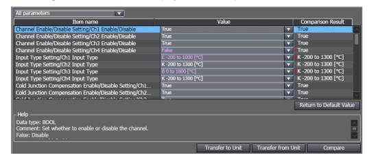
**3** To change the settings in the actual Unit to match those on the Sysmac Studio, click the **Transfer to Unit** Button. To change the settings on the Sysmac Studio to those in the actual Unit, click the **Transfer from Unit** Button.
