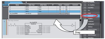
A rung for the SendCmd function block is inserted.
