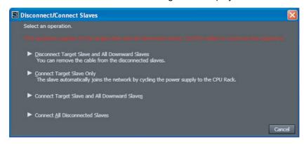
2 Click the Disconnect Target Slave and All Downward Slaves Button. The selected slave and following slaves are disconnected.
