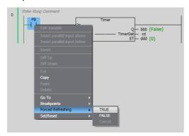
The input or output in the Ladder Editor changes to TRUE or FALSE and the execution condition changes accordingly. An icon also appears by the input or output that represents its current forced value.
