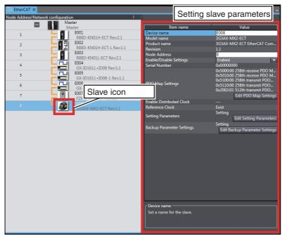
You can edit the parameters for the selected slave. Refer to the *NJ/NX-series CPU Unit Built-in EtherCAT Port User's Manual* (Cat. No. W505) or *NY-series Industrial Panel PC / Industrial Box PC Built-in EtherCAT Port User's Manual* (Cat. No. W562) for information on slave parameters that are not described here.
