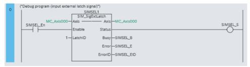
You can check the operation of the debug program by performing a data trace.
