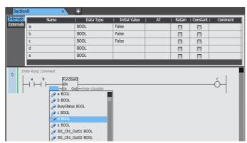
All variables with the correct data type are displayed in the list. The selected variable is entered into the function.
