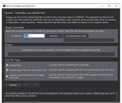
**2** Enter the IP address of the target Controller in the **IP address** field in the **Target Controller** area. If the target Controller is connected directly with a USB cable, enter *USB* for the IP address.
