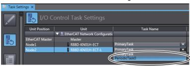
Select the slave/Unit to which you assigned the priority-5 periodic task for the input device or output device in the Axis Basic Settings.
