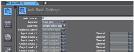
The Axis Parameter Settings tab page is displayed in the Edit Pane. The basic parameters are displayed on the initial display.
