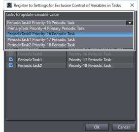
The check boxes of tasks to reference variable are checked by default. To prohibit a task from reading the variables, uncheck the check box.
