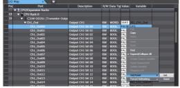
The status of the BOOL device variable changes to TRUE or FALSE and the value in the *Value* Column in the I/O Map changes to TRUE or FALSE.
