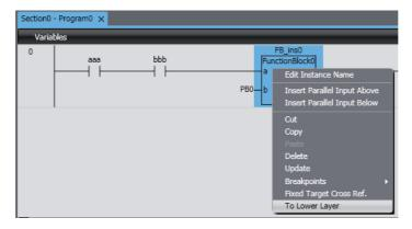
The contents of the function or the definition of the function block is displayed.
