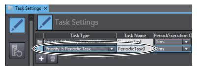
2 In the I/O Control Task Settings under the Task Settings, select the task for the priority-5 periodic task as the task for the slave/Unit assigned to the axis.
