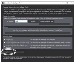
The Controller log is uploaded from the Controller and the directory where the log files were saved is displayed in the **Status** area.
