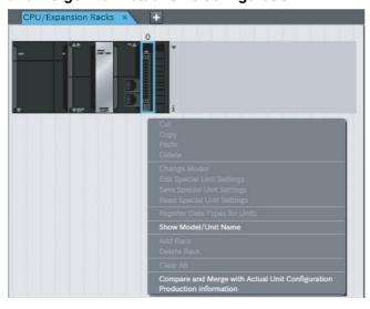
The actual Unit configuration is read and compared with the Unit configuration on the Sysmac Studio. The results are displayed in the Compare and Merge with Actual Unit Configuration Dialog Box.
