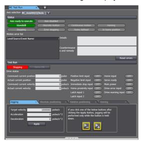
Select the target axis (MC Axis000) at the upper left of the MC Test Run View.
