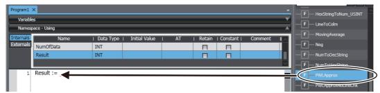
The function or function block is inserted with temporary variables.
