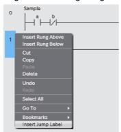
Or, drag a Label under Ladder Tools in the Toolbox to the beginning of the rung.
