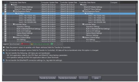
The CPU Rack configuration information is downloaded from the Sysmac Studio to the Controller.
