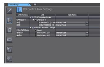
Select the task that should perform I/O refreshing for the registered Unit from the list.
