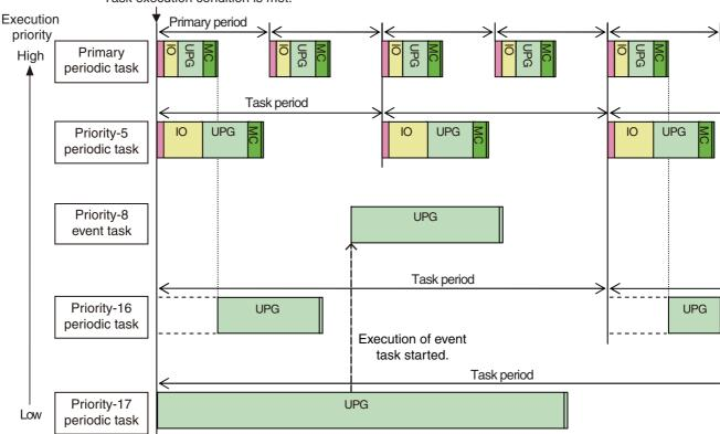
IO: Indicates I/O refreshing (data outputs and then data inputs).
