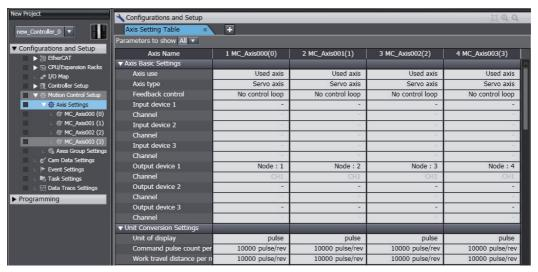
**Note** Each line represents an axis parameter, and each column is for one axis number. All registered axes are displayed. You can collapse the table by axis parameter category.
