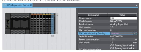
Change the setting to Enabled in the Unit setting item list to enable the Unit again.
