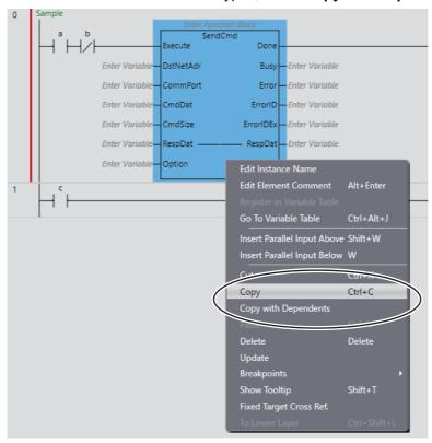
2 Right-click the connecting line where you want to paste the function block instance and select **Paste** from the menu. To paste the function block instance in an OR structure, right-click the circuit part above the location where you want the OR structure and select **Paste** from the menu.
