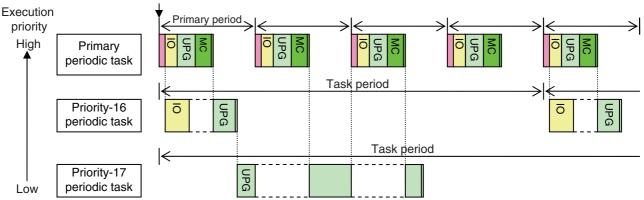
IO: Indicates I/O refreshing (data outputs and then data inputs).
