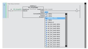
All variables with the correct data type are displayed in the list. The selected variable is entered into the function block.
