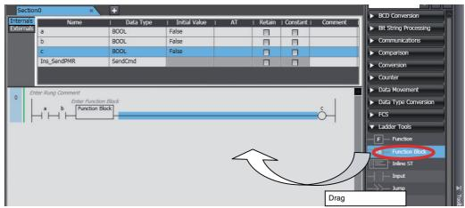
The function block is added to the rung.
