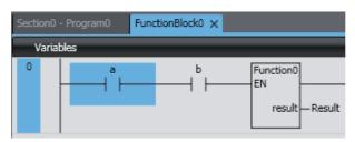
**2** To return from the displayed function or function block definition to the original ladder program, right-click on the function or function block definition and select **To Upper Layer**.
