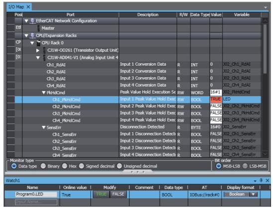
In the Watch Tab Page, register the variables that are assigned to output devices. Refer to 7-2-1 Monitoring on page 7-4 for details on the procedure to register variables in the Watch Tab Page.
