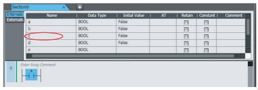
In this case, any variables assigned to the output are not deleted from the local variable table or global variable table.
