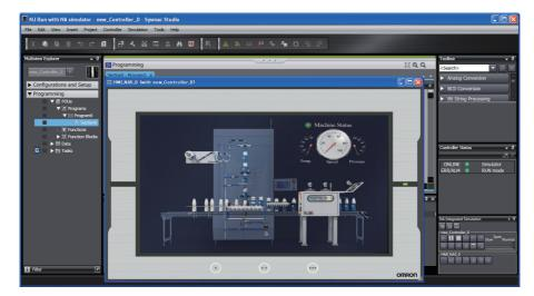
The Simulation Pane has a button that is used dedicatedly for simultaneous simulation of the Controller with an NA-series PT. Refer to *Dedicated Window for Simultaneous Simulation with NA-series PT* on page 7-109 for information on this pane.
