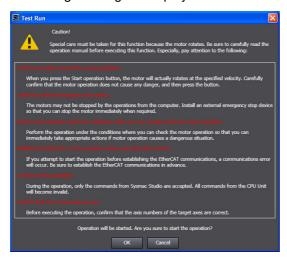
Check the items and then click the **OK** Button. The MC Test Run Tab Page is displayed.
