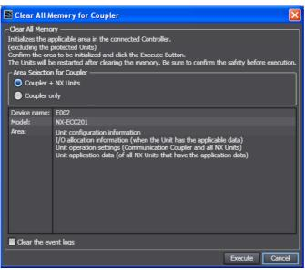
**2** Check the areas to be initialized and then click the **Execute** Button. To clear the event log, select the *Clear the event logs* Check Box. To perform the Clear All Memory Operation for all of the Units, select *Coupler + NX Units* for the *Area Selection for Coupler*.
