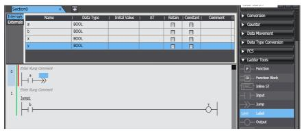
Click Enter Jump Label for the jump circuit part and enter the name of the label to jump to.
