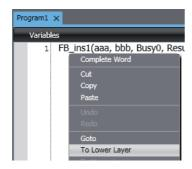
The contents of the function or the definition of the function block is displayed.
